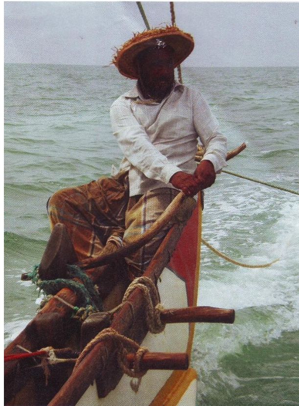
Figure 7. With the oru on the port tack the helmsman controls it with a curved tiller thrust into the rudder/leeboard. (reproduced by kind permission of Mihiri Devendra)
