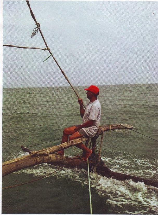
Figure 11. Tuanie Ismail demonstrates how crewmen climb out onto the main outrigger boom to maintain stability. The timber on which he is sitting and which extends beyond the outrigger is the kadise . (reproduced by kind permission of Mihiri Devendra)
