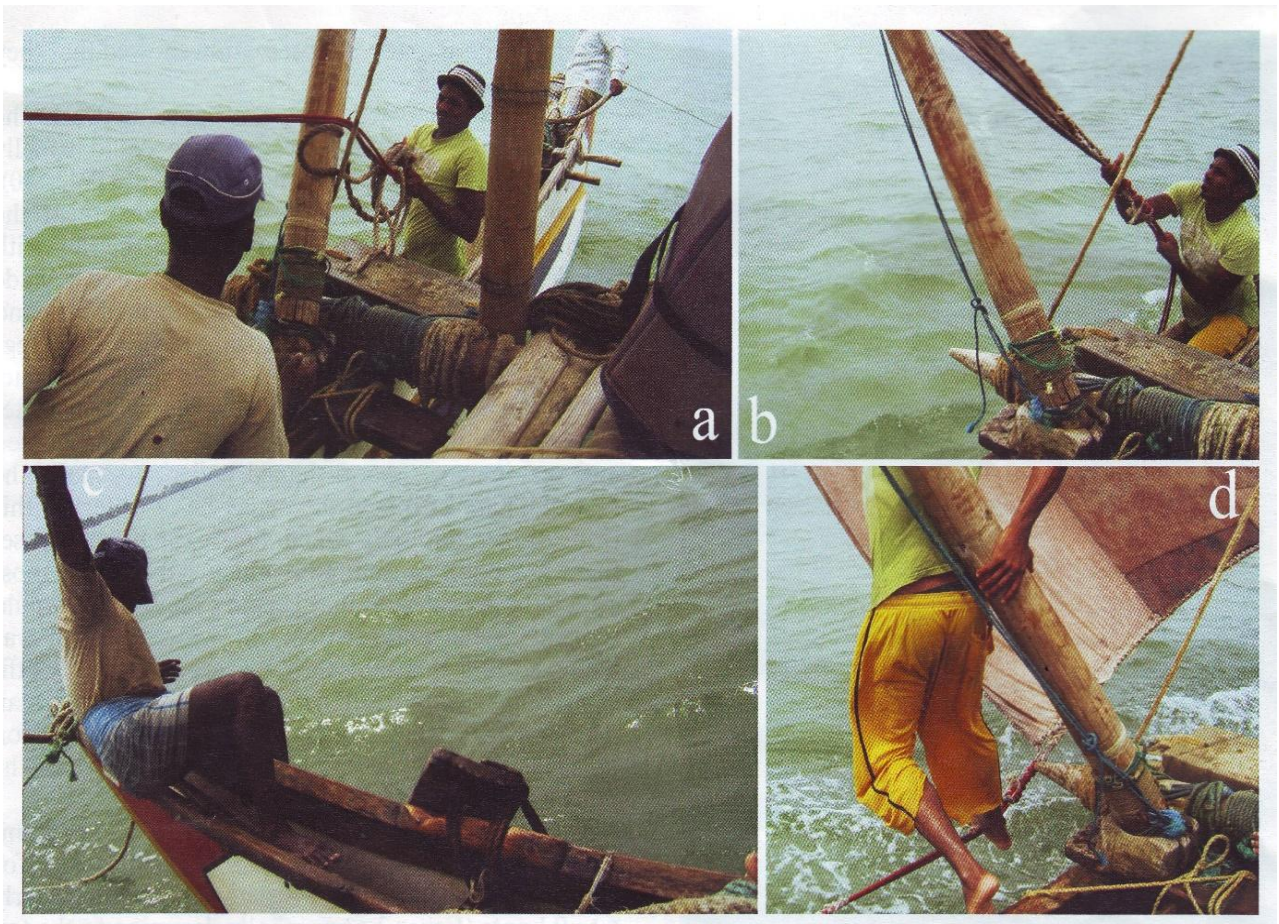
Figure 6. Going about. From top left clockwise: a) having brought the sheet inboard of the sprit, this crewman is gathering it up to pass it back outboard of the sprit to the crewman in the foreground; b) the tack of the sail has been released and the crewman is hauling the sail by the sheet towards the new fore end; c) this crewman is using his body-weight to bowse down the backstay; d) the oru is now picking up speed close-hauled on the starboard tack and the crewman is stamping down on the sheet to bring it under the leeward end of the main outrigger boom where a notch has been cut to receive it. (Gerald Grainge)
