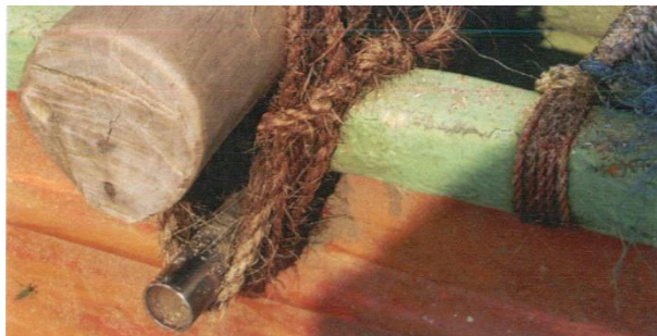
Figure 18. In this podu-oru the anchorage for the outrigger boom is a stainless-steel tube rather than the traditional wooden peg. (Gerald Grainge)
