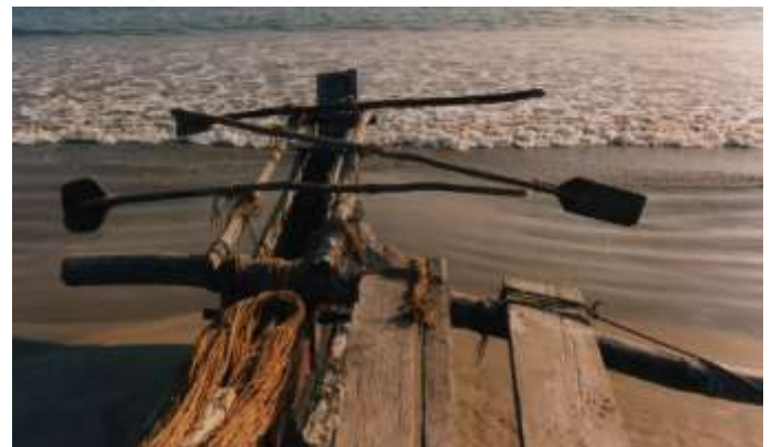
Fig. 20 A mā dāl oru showing the configuration of the oars up forward in the bow. Also visible in the photograph is the extension of the hull-side end of the forward outrigger boom, which allows the shore crew to launch and recover the log boat. From Kapitän, 2009, photo 70
