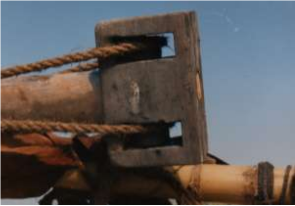
Fig. 26 Another view of the kōvāna , this time with the mast unstopped. Without this rotating block South coast oru hoist their sails with the halyard running through a hole in the top of the mast and do not reverse ends when tacking. Detail from Kapitān , 2009, photo 33b
