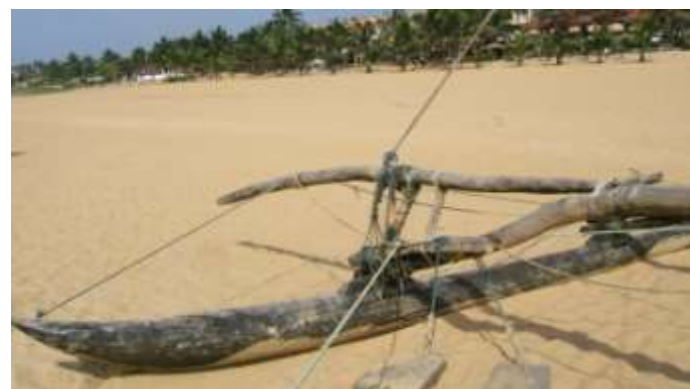
Fig. 12 The kaḍise lashed to the central boom. Also seen are the two humps on the outrigger and the kanhiya in them to which the booms are lashed, together with the stay running to the mast head
