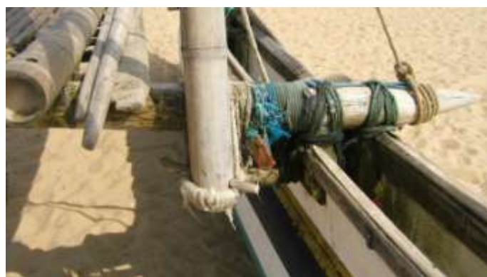
Fig. 13 Reverse view of the central boom shown in Fig. 10, showing the foot of the main mast slung from the central outrigger boom, a feature the West coast oru shares with the South coast oru
