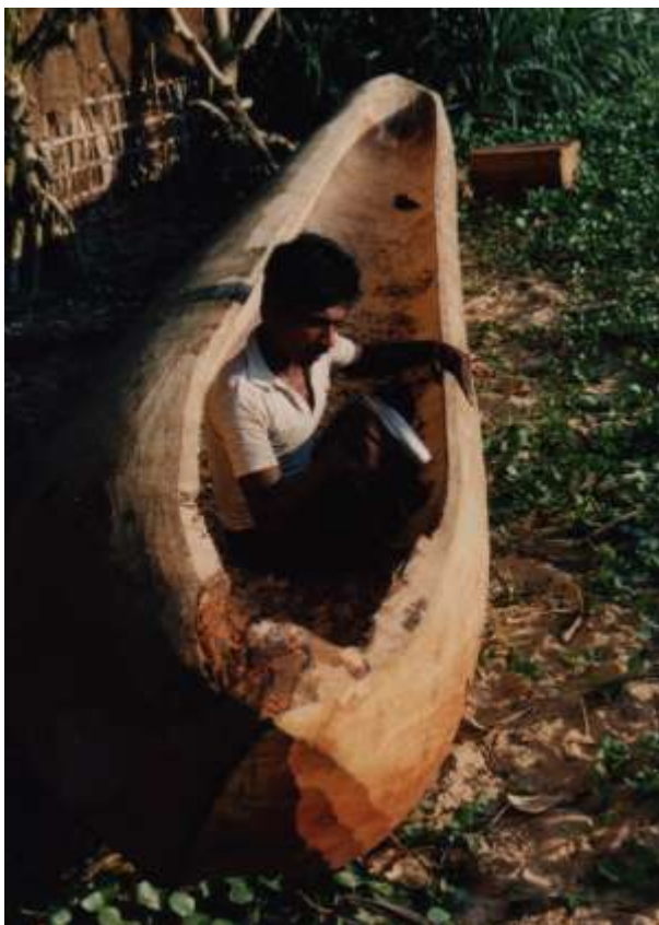
Fig. 7 Hollowing out a logboat hull with an adze. From Kapitän, 2009, Photo 39
