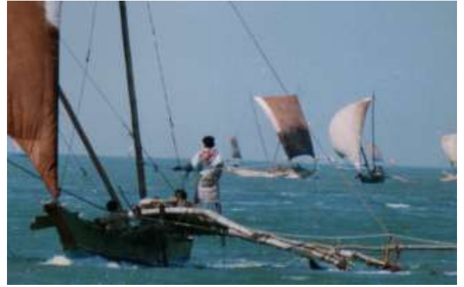
Fig. 14 The crewman standing on the boom is hanging onto the atvāla or lifeline running from the main mast to the vāvarē . From Kapitän, 2009, Photo 77
