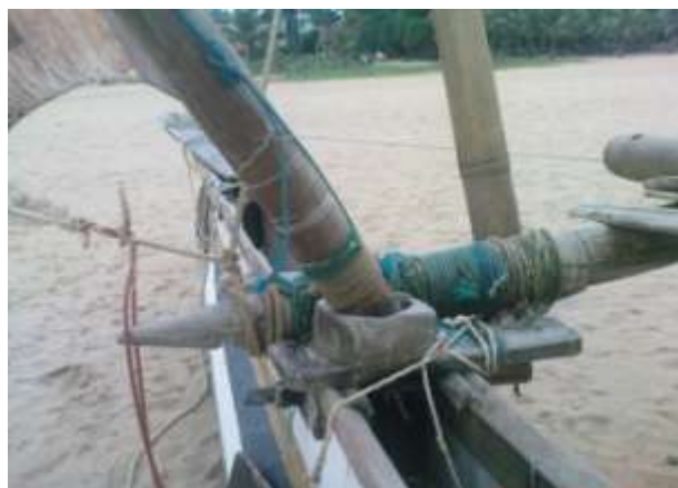
Fig. 10 Detail of the lashing of the central boom of a West coast oru, showing the mast step ( kavaya ) for the secondary mast
