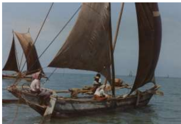
Fig. 11 This photograph of a West coast oru show a palla (rudder plank) at one end of the hull and two at the other, which are changed one for the other when the oru changes tack (Grainge, 2012, 161–2, 166). From Kapitän, 2009, Photo 75
