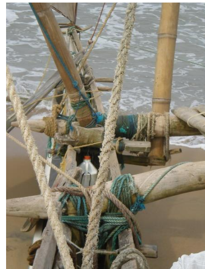
Fig.7. Lashing to an oru . (L to R) A rudder on a grommet, two bamboo sprits (main lashed to a boom), both booms lashed to the hull, and Platform above the booms (Source: Kapitan)
