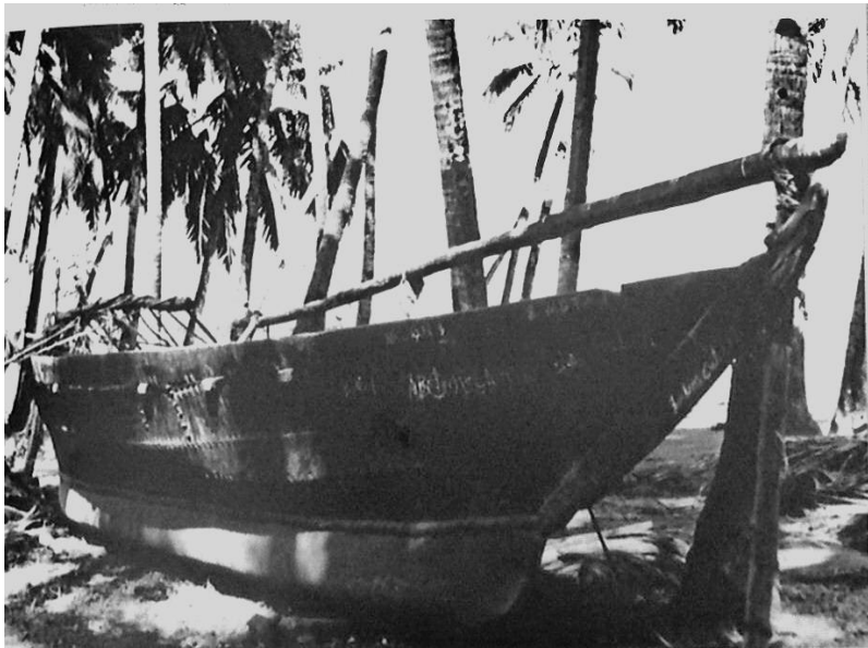
Fig.18. Plank hulled boat with single dugout keel, with sharp bows.
