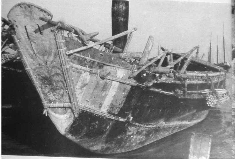
Fig.17. Plank hulled boat with single dugout keel, blunt-ended.
