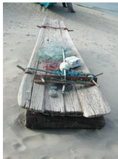
Fig. 5. teppam : pegged-log raft
