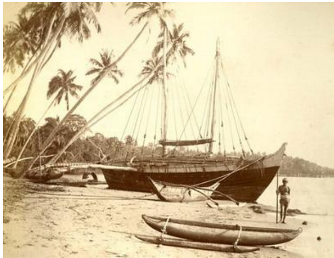
Fig.11. yāthrā dhōni : plank-hulled, seagoing cargo ship with outrigger
