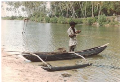
Fig. 8. pilā -oru : outrigger without washstrakes and sails
