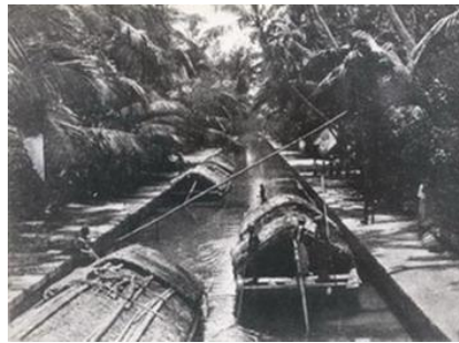
Fig. 7. pāruwa : twin-hulled cargo craft
