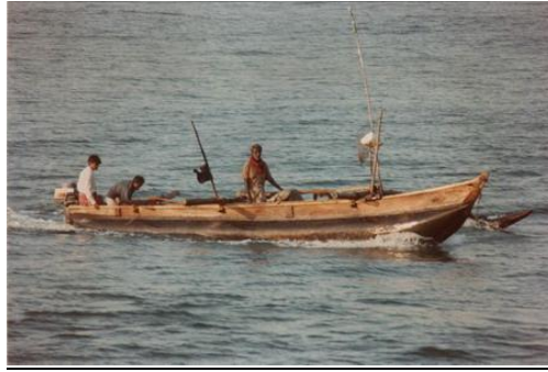
Fig.14. Outboard motor on the transom stern of a mechanized vallam oru
