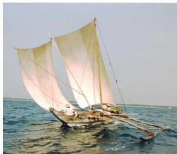
Fig. 9. oruwa : seagoing outrigger craft
