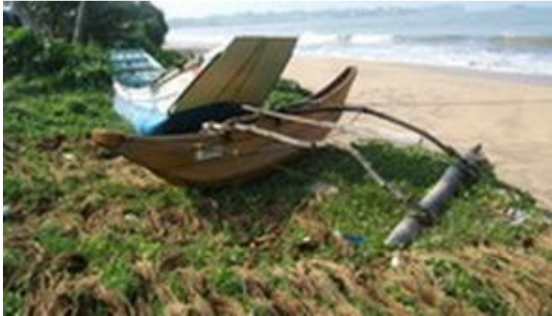
Fig. 15: Small oru with hull and washstrakes moulded as one. Behind: a mā-dāl-pāru of GRP
