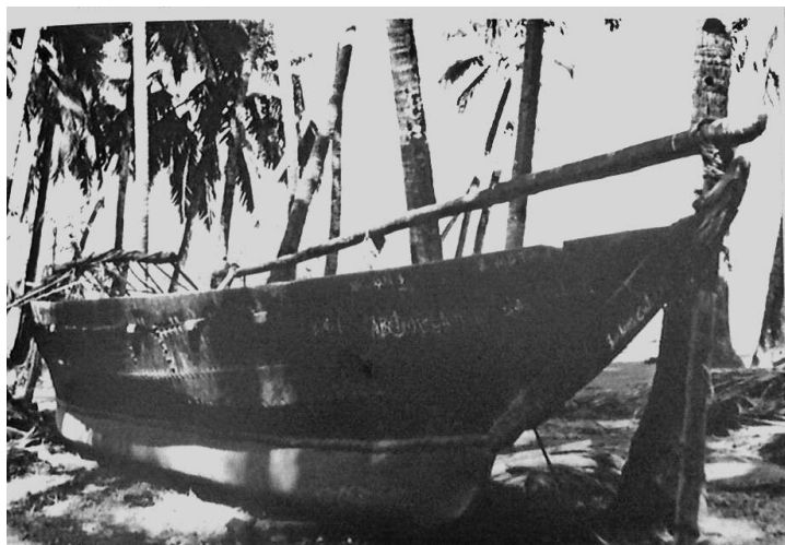
Fig. 8: Boat from Kerala showing dugout keel-log (Source: Hawkins)
